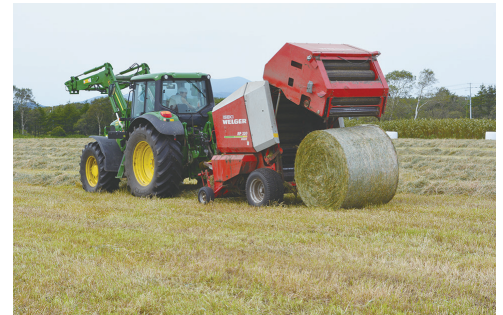
Baling operation by a round baler
